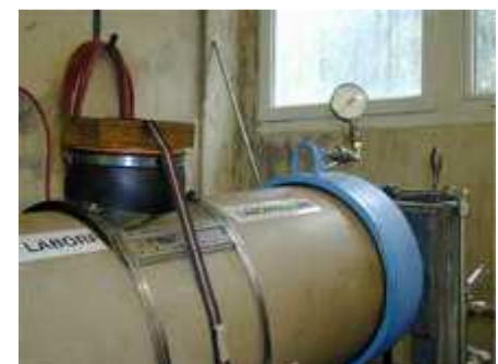
T-flex test on fiberglass pipe
