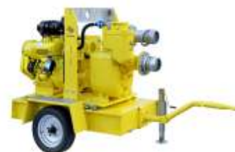
Impianti well point Well point plants
